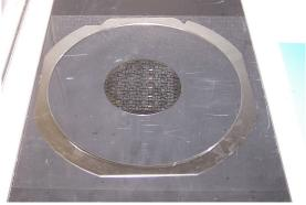
Place the adhesive film on top of the cover sheet/ring/samples (sticky side on the sample).
