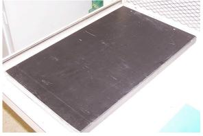
Retrieve the film that you are going to use. Separate the clear cover sheet from the adhesive film. Place the clear cover sheet on the black block and set the adhesive film to the side (with the sticky side up).
