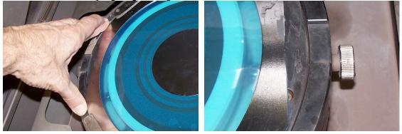
*This is EXTREMELY IMPORTANT!!!* Ensure that the clamping ring and mounting ring are both below the chuck table grinding surface. To confirm this you may use the straight edge of a mounting ring. If the rings are not below the chuck table grinding surface, **DO NOT PROCEED** until they are below the chuck table grinding surface.
