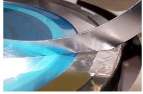
Once the mounting of the rings is complete and the rings have been confirmed to be below the chuck table grinding surface, proceed with the normal grinding procedures.
