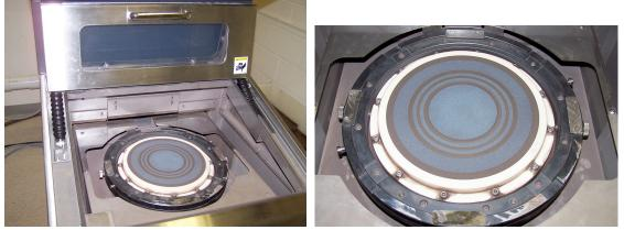
Place the ring with the tape and your sample onto the chuck table. Align the 2 notches on the ring with the 2 alignment pins on the chuck table. Rotate the clamping ring to hold down the ring. From the menu select "Work Size" and set it to 8 inches. Again from the menu select "Work Set" and then turn on the vacuum to the chuck table.
